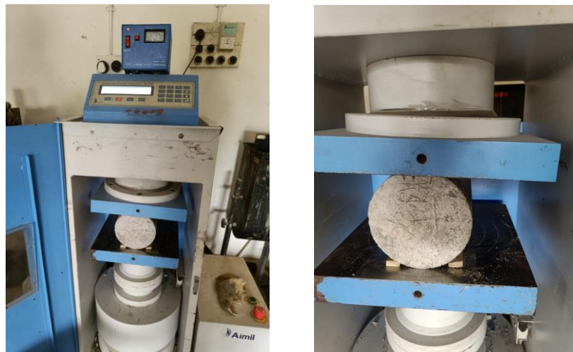
Figure 3 Cylinder Cracked during split tensile strength test
