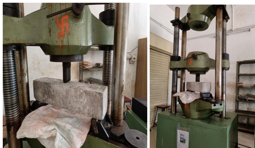
Figure 4: Flexural strength Test Apparatus
