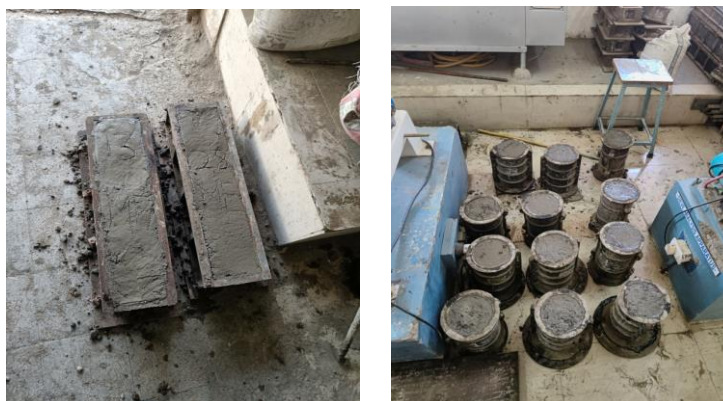
Pic 1: Casted Cube and Cylinders
