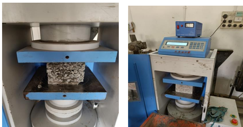
Figure 2: Test performed on concrete cube break after compression
