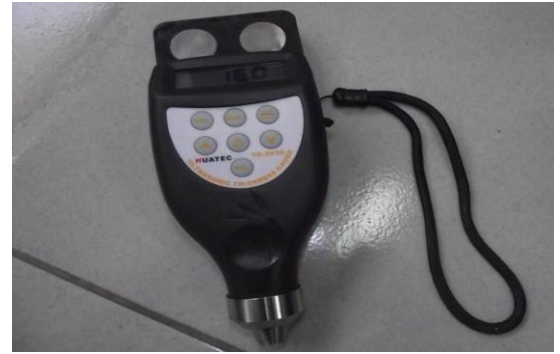
Fig. 3:Diagram for critical cross section Fig. 4: Ultrasonic thickness detector. of tube after deformation.
