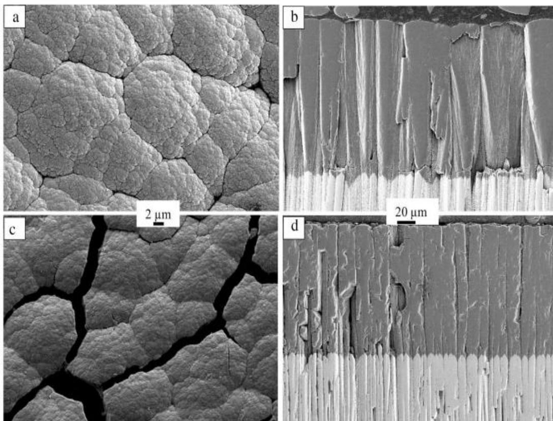
**Fig.4** SEM micrographs taken on the top surface of the EB-PVD alumina coating, before (a) and after (c) the heat treatment at 1100 °C for 30 min, (b) and (d) are the cross-sectional images of the Al<sub>2</sub>O<sub>3</sub> coating after heat treatment.
