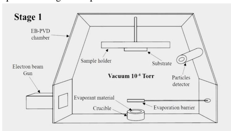
**Fig.1** schematic illustration of the device configuration [4]
