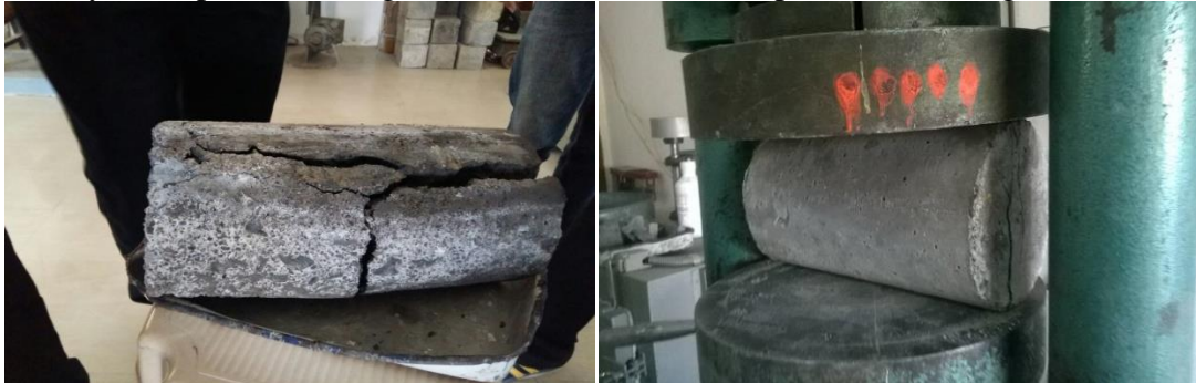
Figure7: Cylinder cracked during split tensile strength test, Split tensile test on cylinder
