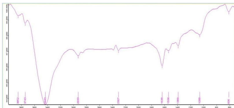
Figure 3: FTIR spectrum of LPA-AgNPs
