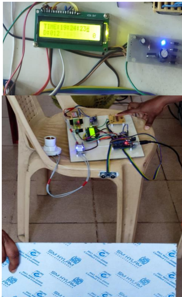
Fig 6.2 real time data measured by Ultrasonic sensor range – indicates the child is sitting in 100cm in front of TV
